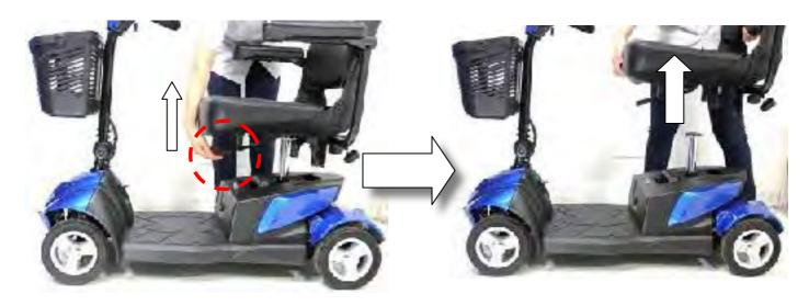
5. Remove the seat by pull the seat rotate lever.
