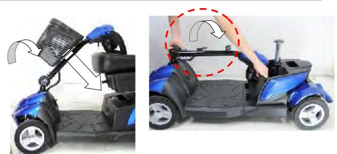
8. Loosen the tiller adjustment knob and fold down the tiller and retighten knob.
