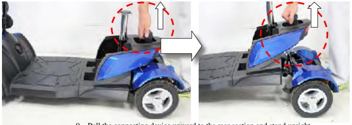
9. Pull the connecting device upward to the rear section and stand upright.
